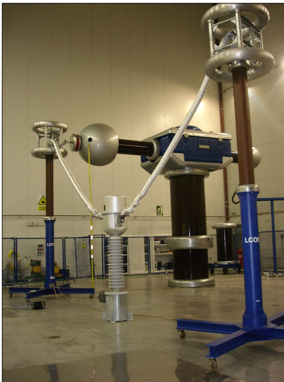
➤ Figure 3 – Picture of combined transformer. RIV Measurement.
